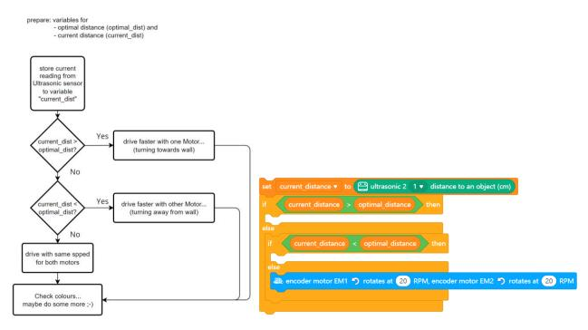
In these statements, the robot would only drive straight on, if optimal and measured distance are identical... and the ultrasonic sensor measures with an accuracy of 0.1 cm. How likely is an identical value of optimal and measured distance? This could be improved by using the deviation from the optimal position and including this into the conditional statements... allowing a range of values for driving straight on:
