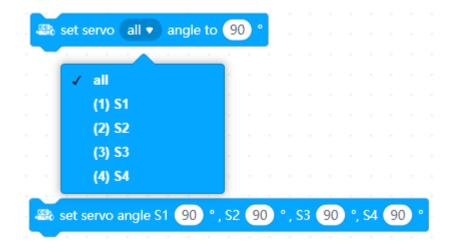
Servo Motors rotate between 0 and 180 degrees; however, this can be limited by the mechanical construction they are used with. So, Students should test the values they will use with care!
