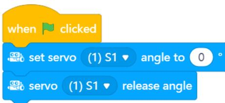
*This will position the servo to the starting position. So as soon as you attach the gate, it will be in the correct position.*
