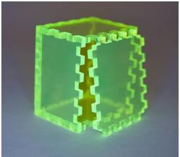
This technique produces a much stronger joint compared with simply gluing two pieces together in what is known as "butt joint". Because of this, it is often utilized in projects with structural requirements. The properties of finger joints will be further discussed in Section 3.
